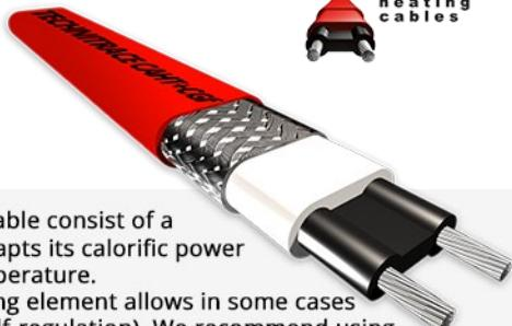
CAHT high temperature self-regulating heating cable consist of a heating semiconductor plastic element which adapts its calorific power (W/m) on each point depending on the local temperature.
