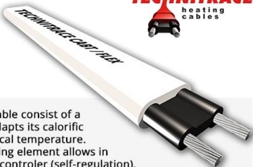
CABT low temperature self-regulating heating cable consist of a heating semiconductor plastic element which adapts its calorific power (W/m) on each point depending on the local temperature. This intrinsic feature of the semiconductor heating element allows in some cases to dispense of using a thermostatic controller (self-regulation).
