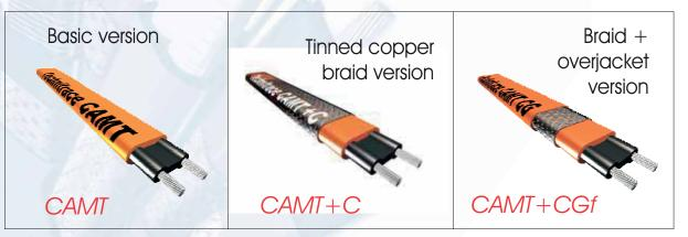
Do not use the CAMT heating cable on plastic pipe. It is imperative to comply with FIQ93 operating instructions. Warranty maxi exposure temperature : power ON = 85°C / power OFF 125°C. Maximum maintenance advised temperature : 65°C. Beyond these exposure temperatures use control thermostat.
