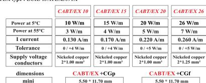
Printing: CABT/Ex - Ex e IIC T6 Gb - Ex tb IIIC T85°C Db - IP 66/67 Temperature range: -50°C < Ambiant Temp <+65°C.
